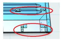
**TIP:** Drill the lower holes on an angle into the thicker part of the model so the edge doesn't break.
