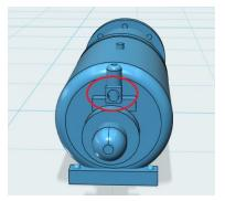
9) Glue the large brake clevis to the K brake part and then mount on the bracket pad. The cylinder has 2 pads on it. The piston rod and clevis point to the "B" end of the car.
